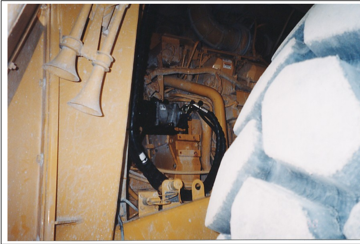
Compressor showing set-up and hose routing.
